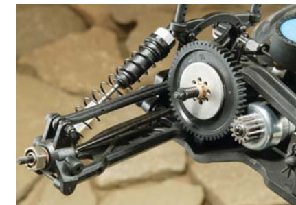
The rear suspension absorbs the roughest bumps, and the slipper clutch helps to minimize the risk of damaging the transmission.
