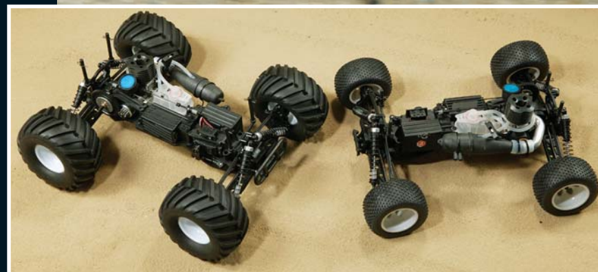
The MT3 and TRII have the same MG10 chassis but different tires and bodies.
