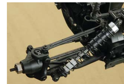
The MG10 chassis has many mounting places for the camber-link mounts and the shocks. This allows drivers to adjust the suspension geometry to meet their needs.
