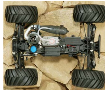
The wide-stance MG10 chassis offers a sealed radio box and a low center of gravity.
