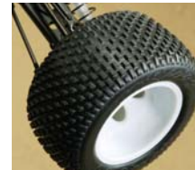
The TRII's CEN medium-compound rectangular-lug tires provide great traction for racing.
