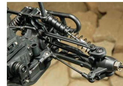
The innovative front steering setup eliminates bump-steer, and the internal outdrives don't have output cups that wear out.
